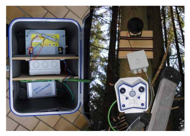
Figure 1: Left: Weatherproof, isolated and lockable box of digital video camera system with open lid: at the top the battery, in the middle the voltage converter and at the bottom NAS (Network Attached Storage). Right: Digital video camera (at the bottom) with infrared illuminator (at the top) and twilight switch for the infrared illuminator (in the middle). The infrared illuminator is attached to a small board so that it can be adjusted easily. This board is fixed with strips to a tree trunk.
