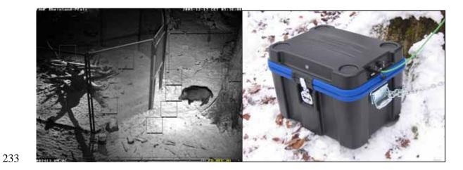
Figure 2: Left: Screen print of the black-and-white night lens of the digital video camera with motion detection windows (rectangles with dotted lines). These motion detection windows evaluate changes in pixel brightness between two succeeding live images. Right:
